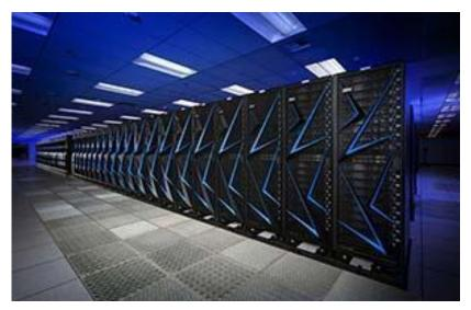
Figure 12. Sierra is an IBM supercomputer sited at Lawrence Livermore. Containing 17,280 NVIDIA GPUs and 8,640 IBM P9 CPUs, Sierra is capable of 125 petaFLOPS. (LLNL)
