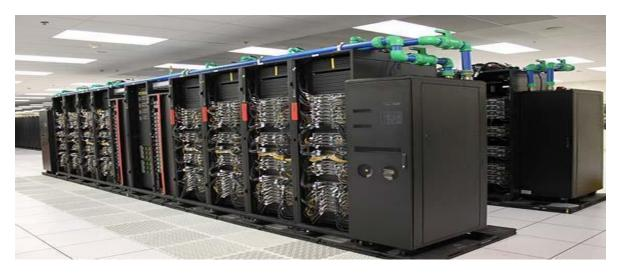
Figure 2. CT systems are supercomputers built from commodity parts. The pictured Magma system at Lawrence Livermore National Laboratory has 1,544 Intel Cascade Lake CPUs and achieves 5 petaFLOPS. (LLNL)
