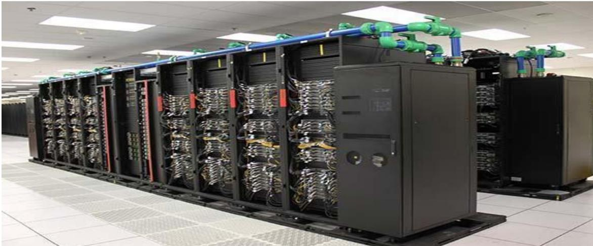
*Figure 2. CT systems are supercomputers built from commodity parts. The pictured Magma system at Lawrence Livermore National Laboratory has 1,544 Intel Cascade Lake CPUs and achieves 5 petaFLOPS. (LLNL)*
