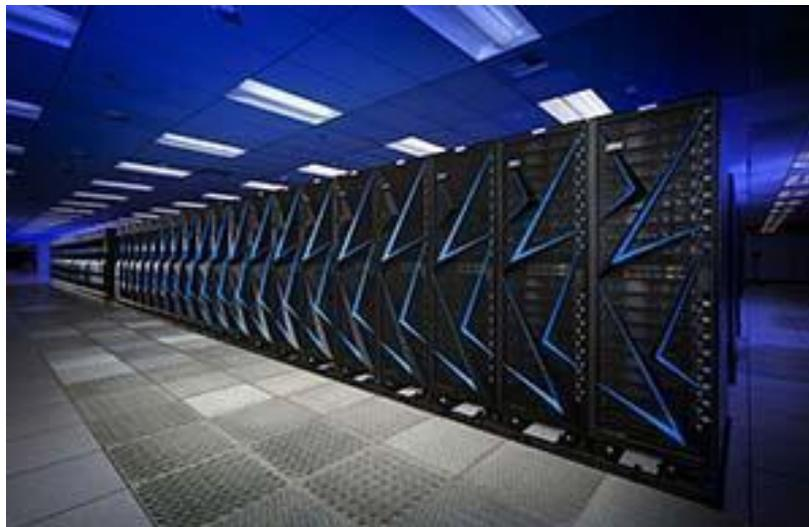
*Figure 12. Sierra is an IBM supercomputer sited at Lawrence Livermore. Containing 17,280 NVIDIA GPUs and 8,640 IBM P9 CPUs, Sierra is capable of 125 petaFLOPS. (LLNL)*
