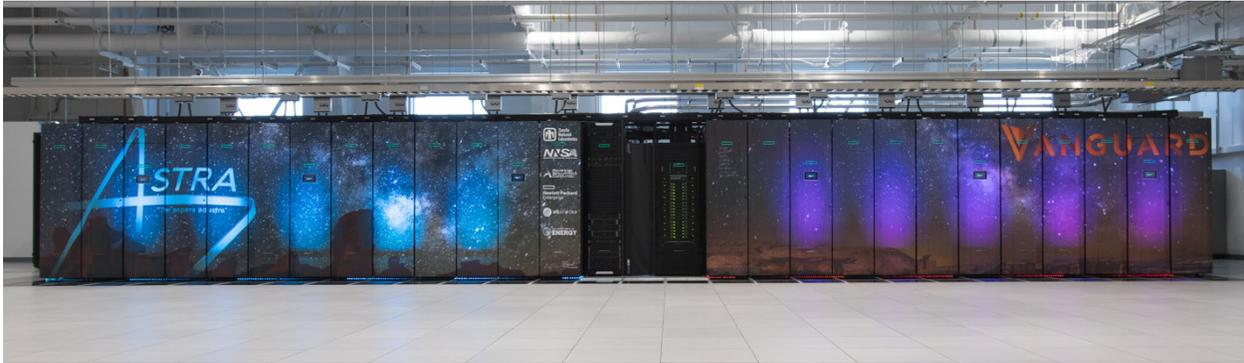
*Figure 4. Vanguard Astra, ASC's first at-scale advanced architecture prototype system and the first petascale Arm-based supercomputer.*
