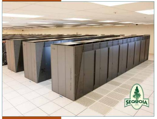
ASC Sequoia—The 20 PETAFLOP/S (QUADRILLION FLOATING OPERATIONS PER SECOND), THIRD-GENERATION IBM BLUEGENE SYSTEM—IS NOW UNDERGOING ACCEPTANCE TESTING AT LAWRENCE LIVERMORE NATIONAL LABORATORY.
