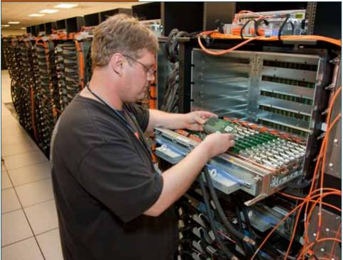
ABOVE: THE PETASCALE HEAT EXCHANGER, WHICH IS PART OF THE COOLING SYSTEM FOR SEQUOIA.
