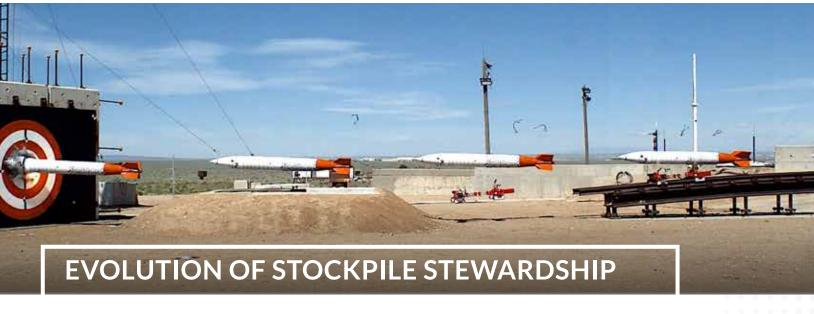
A B61-12 test unit strikes a target during a complex forward ballistics test. The test, which mimicked a high-speed accident, allowed engineers to examine the weapon's safety features. (SNL)
