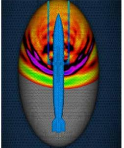
Simulation using the structural dynamics (SD) component of the SIERRA multiphysics code, depicting structural response for the B61-12 to acoustic loading. (SNL)
