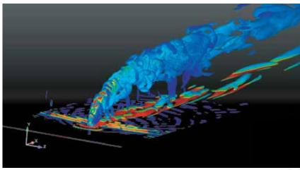
Iso-surfaces of Q-Criterion colored by eddy-viscosity from a Hybrid RANS-LES simulation of a jet-in-crossflow flow field. The image shows the complex interacting vortex structures in the flow field. The algorithms were influenced by information on new hardware changes. (ASC Computing Strategy, 2013).
