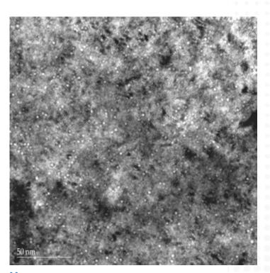
Helium bubbles in a Transmission Electron Microscopy (TEM) image of an aged plutonium sample. These bubbles affect the strength, compressibility, and other properties of the material. (LLNL)
