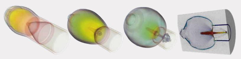
The evolution of a shaped charge jet as simulated by MARBL.
