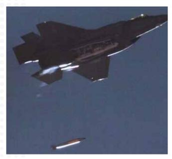
An F-35A Lightning II opens its bomb bay doors and drops a mock B61-12 at SNL's Tonopah Test Range.
