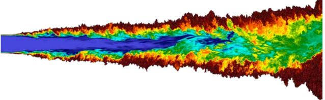
Chaotic mixing of fluids in a turbulent jet using several billion cells. The Sierra platform has reduced the time required for these high-resolution simulations from more than a month to the span of two or three days. Rather than one-off calculations, these simulations can now be run as part of routine studies to better understand the complex flow features of turbulent mixing and validate engineering models.
