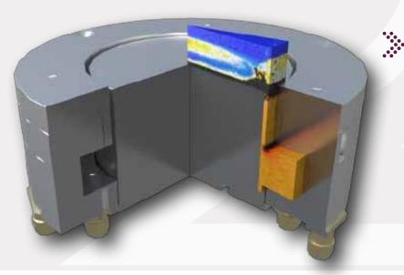
Experimental CAD geometry as fielded on the Z pulsed power X-ray facility with an overlay of a plasma generated in an EMPIRE simulation. The extreme-scale computational resources of Trinity and Sierra are necessary to model the complex dynamics generated by the X-ray generation from the SNL Z facility.
