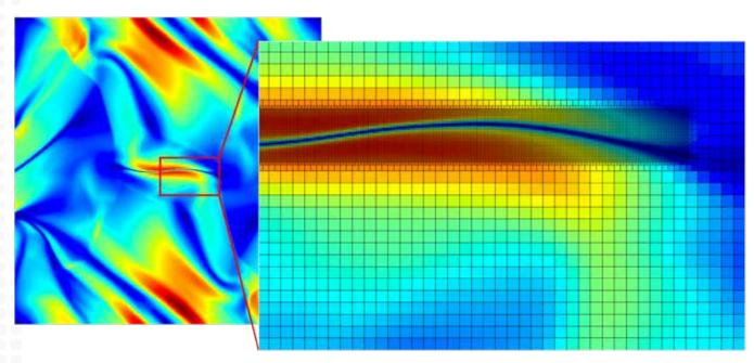
Magnetohydrodynamic (MHD) simulation with LANL xRAGE multi-physics code under the Eulerian Applications Project. MHD simulations are important to many inertial confinement fusion (ICF)/highenergy-density (HED) and stockpile applications. The simulations continue to be improved to support modeling experiments using laser-driven hohlraums.
