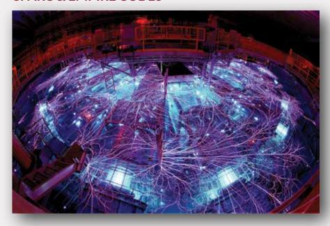
Sandia's Z Machine oncentrates electrical energy and turns it into short, enormously powerful pulses to generate X-rays and gamma rays.
