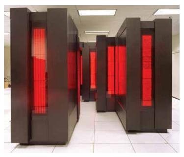
The innovative Connection Machine, CM-5, was the first parallel computer used for stockpile related purposes at LANL. It was built by the Thinking Machines Corporation. (LANL)
