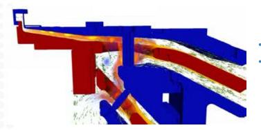
EMPIRE simulation of Sandia Z-accelerator experiment showing electron density in the magnetically insulated transmission line using Kokkos as the performance portability layer.
